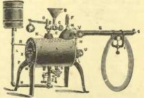
end of the arm G should be opened for a time to blow the air out of the boiler and arm, when about to commence vulcanising. The steam from this vulcaniser is absolutely dry, being taken from a dome after the manner of a horizontal boiler. By a sheet iron jacket, the heat from the burner is concentrated into heating the boiler, without unduly heating the surrounding room, the hot air, finally passing out through the holes at Y.
