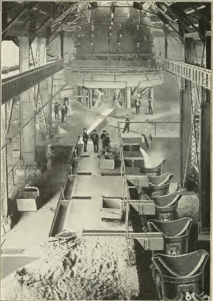
Running molten iron from the blast furnaces into ladles which transport it to the steel mills where it is made into steel.
