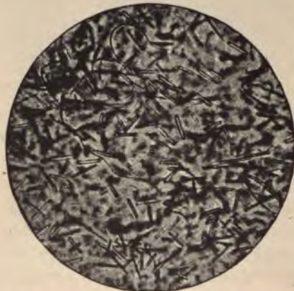
A slice of volcanic glass under the microscope, showing well-developed microliths. (After Cohen.)
