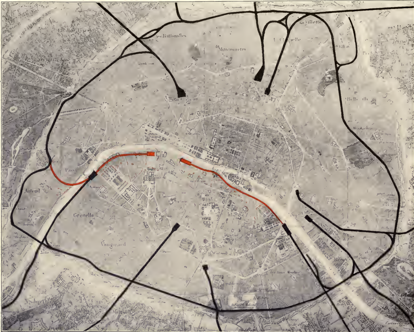
PLATE 58. STEAM RAILROAD MAP OF PARIS SHOWING, IN RED, TWO STEAM LINES EXTENDED (ELECTRIFIED) INTO INTERIOR OF THE CITY. 1900.
