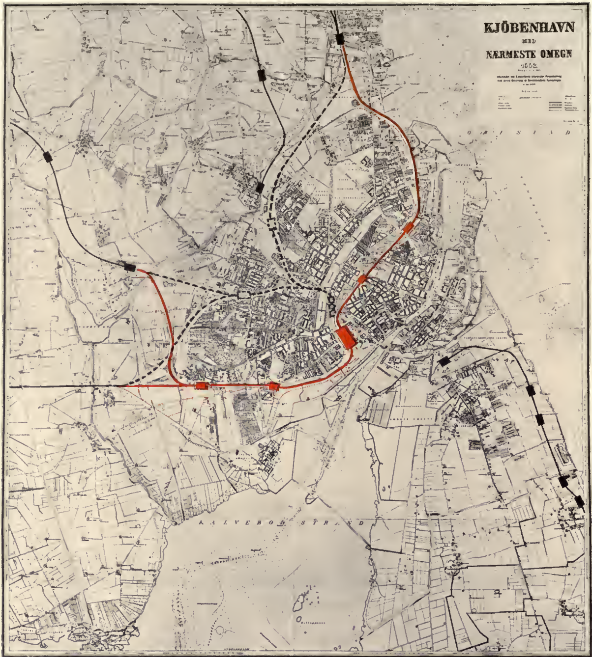
PLATE 66. MAP OF COPENHAGEN, SHOWING, (a) ABANDONED STEAM TERMINAL LINES; (b) SUBSTITUTED THROUGH-ROUTE SYSTEM NEARING COMPLETION, 1913.
