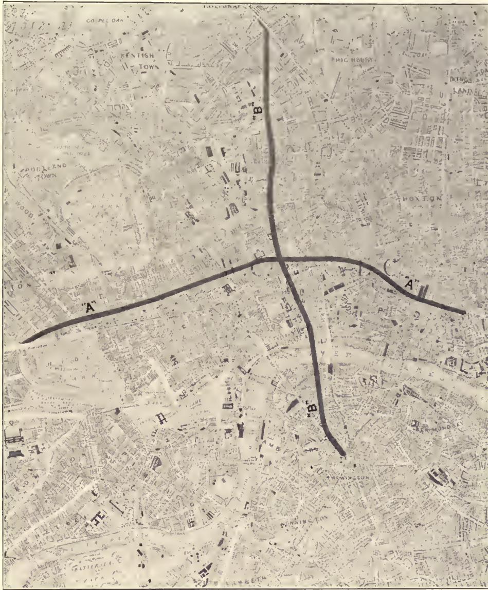
PLATE 55. MAP OF STREET-AND-RAILROAD ARTERIES SUGGESTED FOR LONDON BY ROYAL COMMISSION ON LONDON TRAFFIC, 1905.
