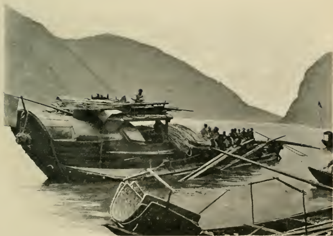
Salt Junk, about 70 Tons, with Screw-oars or "Yuloes" alongside, moored near Entrance to Ichang Gorge: bound down River, Mast lashed alongside.
