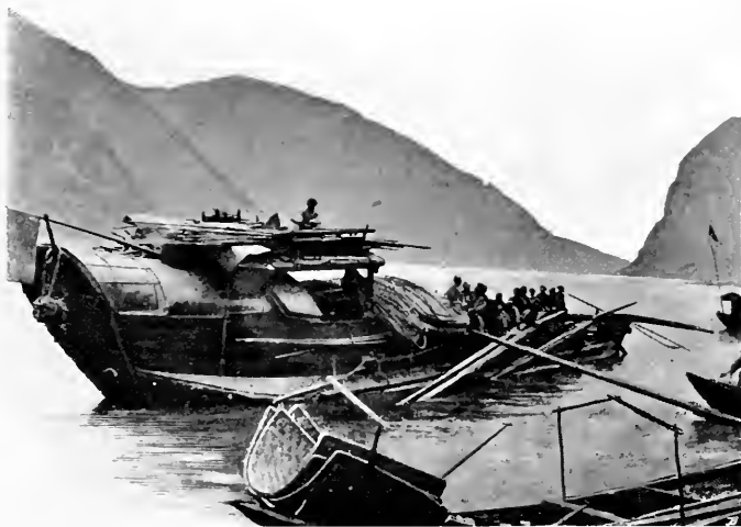
Salt Junk, about 70 Tons, with Screw-oars or "Yuloes" alongside, moored near Entrance to Ichang Gorge: bound down River, Mast lashed alongside. [To face p. 222.]
