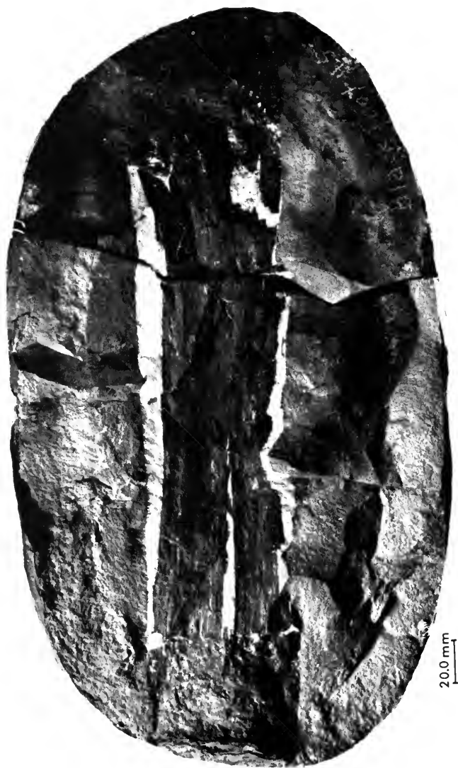
FIG. 1. Broken horizontal surface of concrete from black shale over Springfield Coal (No. V), Pike County, Indiana. Fossil wood, with well-preserved cell structure, lies along the center outlined by the white calcite veins. The black zones extending from the fossil wood to the concrete's exterior represent the extremities of the wood that were completely degraded after the concreting process was well advanced. Note the sharp boundaries with concrete matrix. Lighter colored areas in the concrete matrix are pyrite concentrations adjacent to the fossil wood and as a "halo" closer to the concrete surface.
