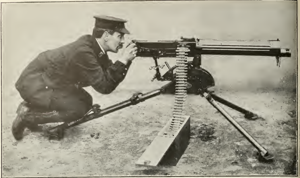
VICKERS' LATEST QUICK-FIRER. Firing 600 rounds per minute.
