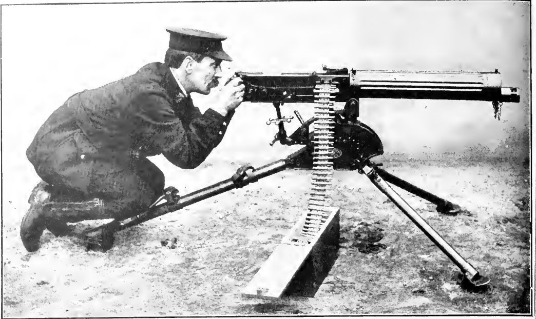
VICKERS' LATEST QUICK-FIRER. Firing 600 rounds per minute.
