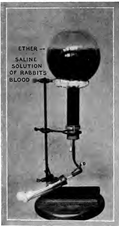
APPARATUS FOR THE PREPARATION OF CULTURE MEDIUM FOR THE GROWTH OF MENINGOCOCCI.
