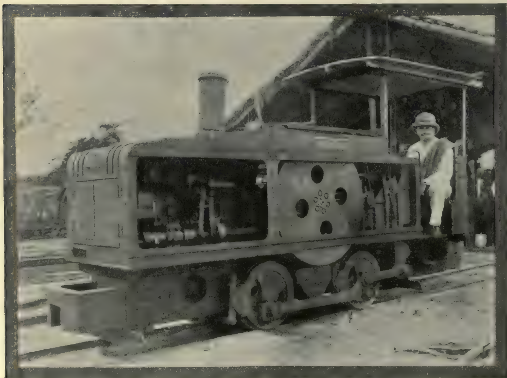
GERMAN LIGHT PETROL-DRIVEN ENGINE CAPTURED AT KILWA.
