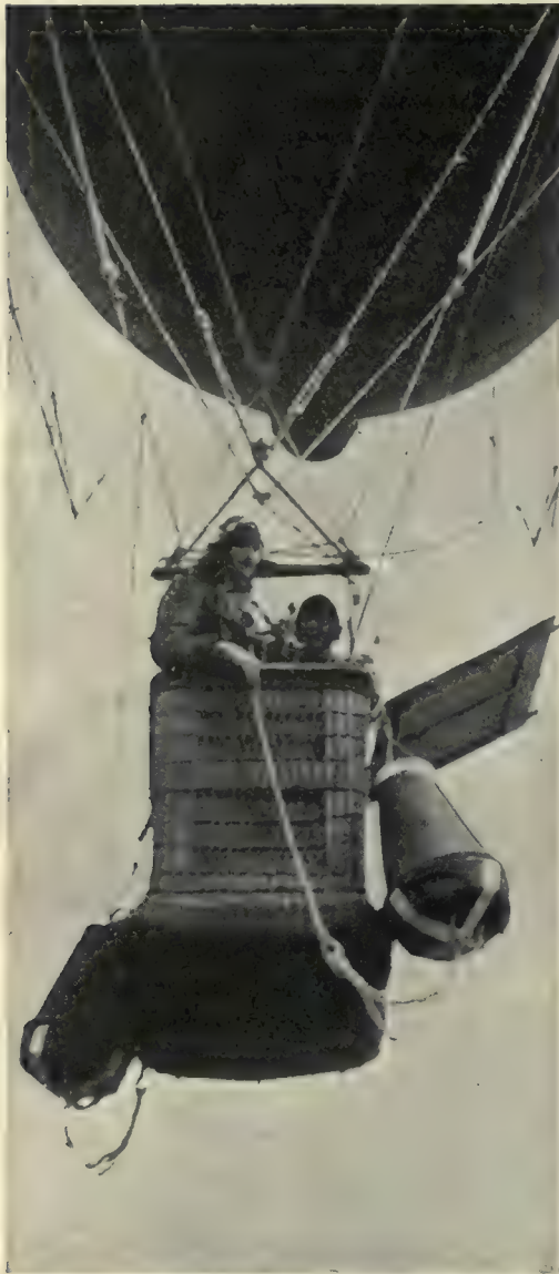
KITE BALLOON WITH PARACHUTES ATTACHED.
