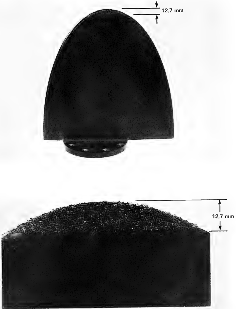
Figure 8 - Overall and Closeup Views of 600 Micron Roughness Applied to the Parent Foil Pressure Side
