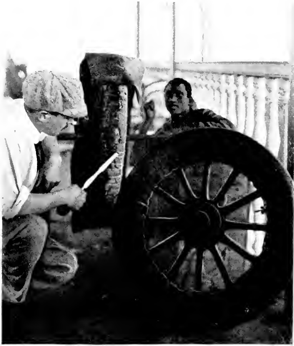
Showing how we repaired tyres with raw hide and rubber
