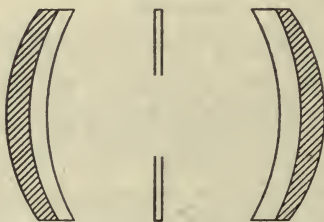
*FIG. 64. DOUBLE COMBINATION LENSE
