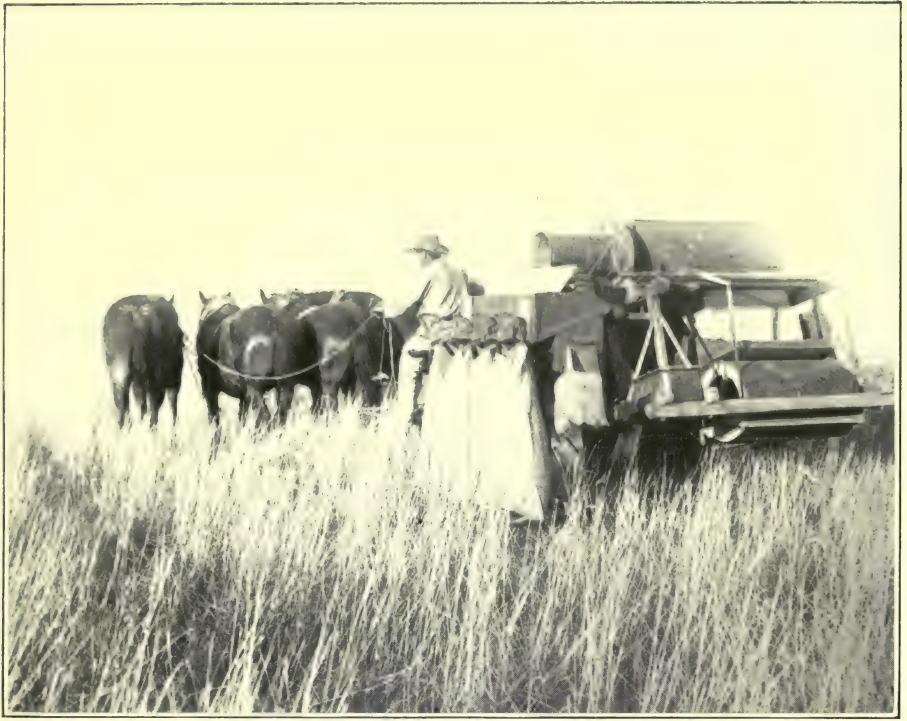
AUSTRALIAN-MADE STRIPPER HARVESTER AT WORK. THIS MACHINE STRIPS, THRESHES, CLEANS, AND BAGS AT ONE OPERATION.
