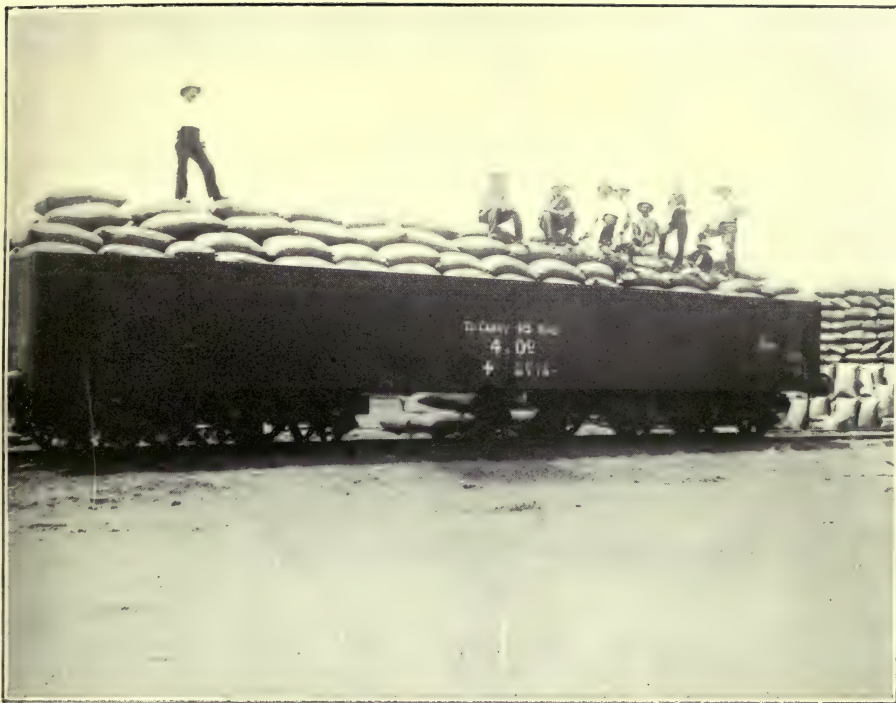
45-TON CAPACITY WHEAT TRUCK.
