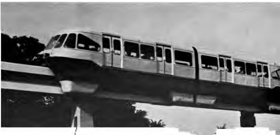
(Below) Alweg supported monorail train on the trial track at Cologne-Fühlingen. (Photo: Alweg)
