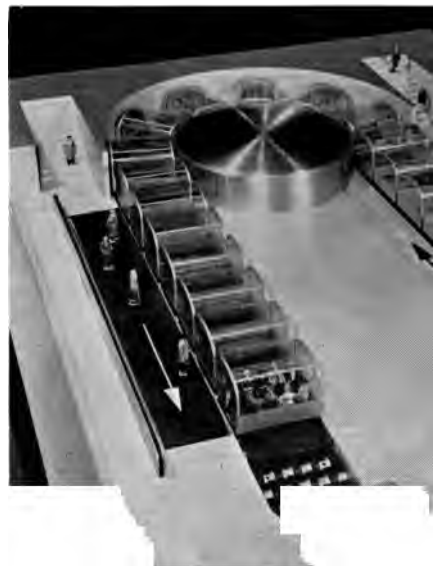
Close-up of part of scale model Carveyor system, showing moving loading platform at station and, in foreground, bank of acceleration rollers. (Photo: Stephens-Adams Mfg. Co.)
