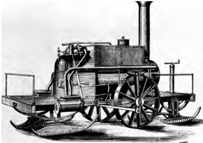
(Above) Ice locomotive built by Nathaniel Grew for service on Russian lakes and rivers. (Photo by courtesy of "The Engineer")
