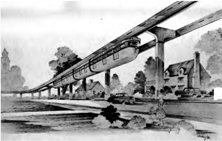
(Above) Gibbs & Hill Inc. proposal for a split-rail suspended monorail system. (Drawing: Gibbs & Hill Inc.)
