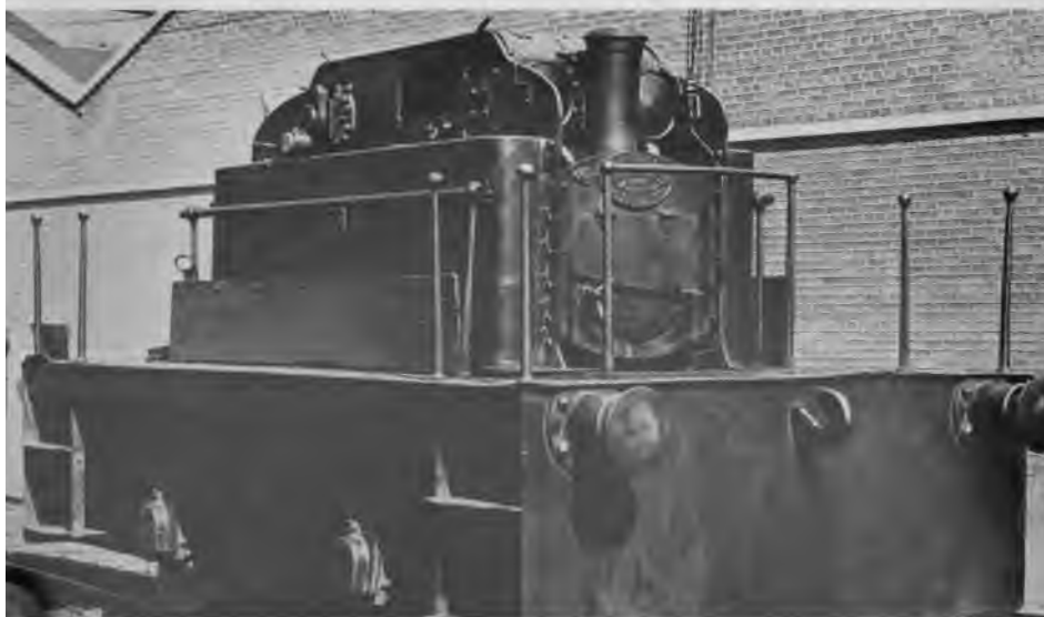
(Below) Narrow-gauge Geoghegan locomotive mounted in a "haulage wagon" to enable it to work over broad-gauge track at the Guinness Brewery in Dublin. (Photos: Arthur Guinness Son & Co. (Dublin) Ltd.)
