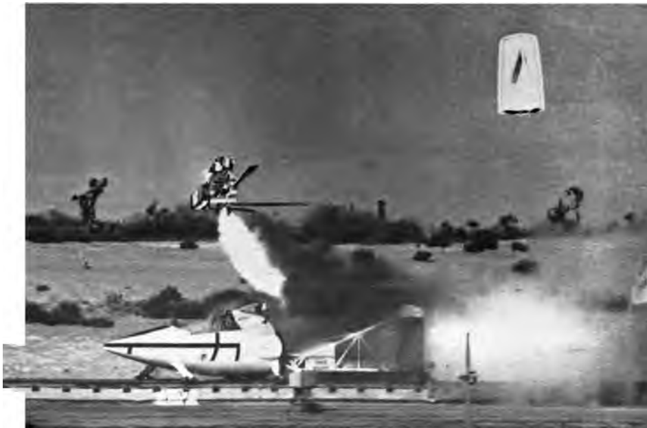
(Below) The Snort track at Inyokern China Lake, California, in use. The pilot's seat is being ejected from a mock-up of the X-15, the aircraft built to fly out of the atmosphere into the fringes of space and return, carrying the first man into space. (Photo: U.S. Air Force)
