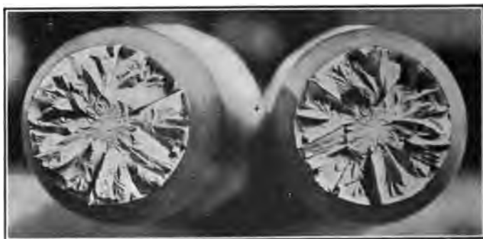
FIG. 20 TEST PIECE RUPTURED UNDER TENSION; FRACTURE ORIGINATED ALONG THE AXIS
