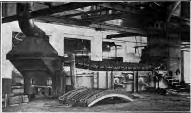
FIG. 6 TYPICAL AIR FURNACE
