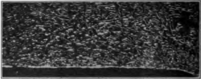
FIG. 9 PHOTOMICROGRAPH OF FIELD AT a , FIG. 8 (60 MAGNIFICATIONS), SHOWING DISTURBANCE OF CRYSTALLINE STRUCTURE DUE TO THE USE OF A DULL HOB IN TOOLING
