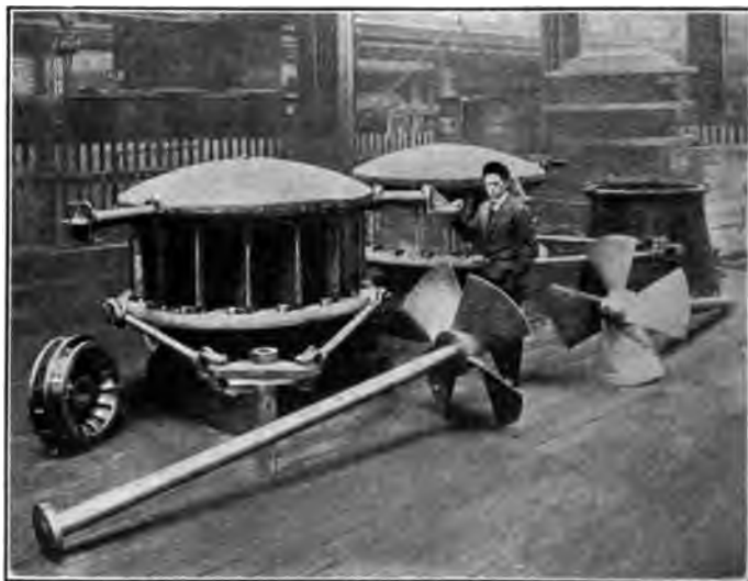
FIG. 3 ONE OF THE FIRST COMMERCIAL APPLICATIONS OF THE NEW "SUCTION" TYPE OF RUNNER DESIGNED IN 1916
