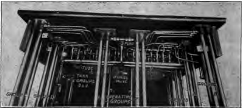
FIG. 8 VIEW UNDERNEATH MODEL NO. 3 OF HARRIS HYDRAULIC BALANCED LIFT, SHOWING PLUNGERS, PIPING CONNECTIONS, ETC.
