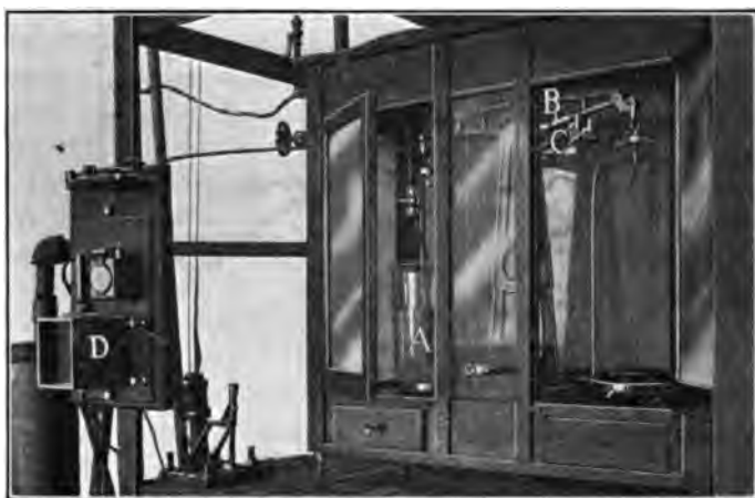
FIG. 2 SCALES FOR WEIGHING GASOLINE, AND ELECTRICAL EQUIPMENT FOR STARTING AND STOPPING TESTS
