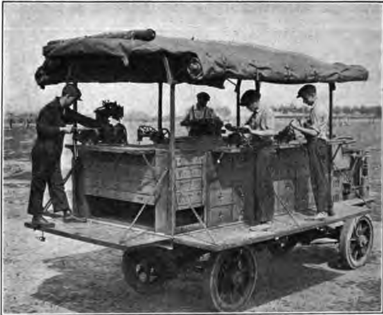
FIG. 8. ORDNANCE MOBILE REPAIR SHOP
