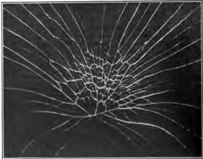
FIG. 4 DEVELOPMENT OF THE FRACTURE RESULTING FROM A SHOCK ON A THIN SHEET OF GLASS
