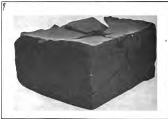
FIG. 17. FRACTURE OF A CAST IRON BLOCK
