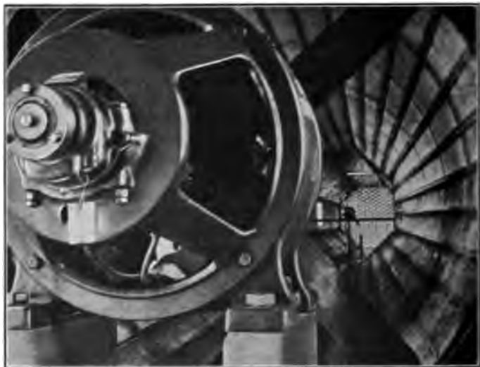
FIG. 1 AIR FAN AND TEST GENERATOR MOUNTED IN WIND TUNNEL
