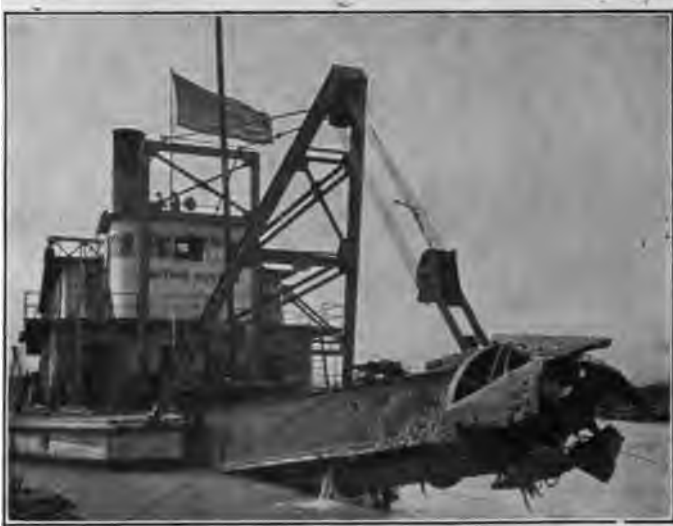
FIG. 4 THE DREDGE Captain Huston , USED IN THE EXCAVATION OF THE NEW ORLEANS INDUSTRIAL CANAL
