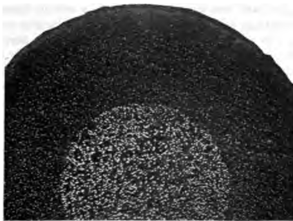
FIGS. 36 AND 37 BARS MAGNIFIED SEVEN DIAMETERS TO SHOW CARBON DISTRIBUTION
