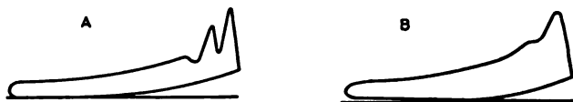
FIG. 1 FULL-LOAD INDICATOR CARDS OF ENGINE RUNNING (A) ON KEROSENE AND (B) ON GASOLINE (200-LB. SPRING)
