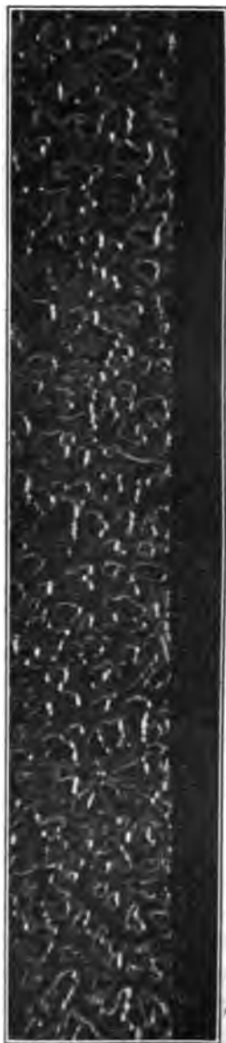
FIG. 11 PHOTOMICROGRAPH OF EDGE b , FIG. 8 (90 MAGNIFICATIONS), SHOWING THAT A SHARP TOOL WITH SUFFICIENT RAKE WILL NOT DISTURB THE CRYSTALLINE STRUCTURE
