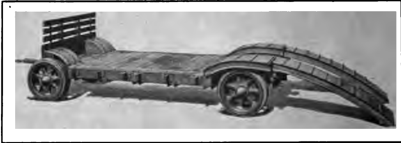
FIG. 7 ARTILLERY 10-TON TRAILER FOR TRANSPORTING TRACK-LAYING TRACTORS, SMALL TANKS, OR GUNS
