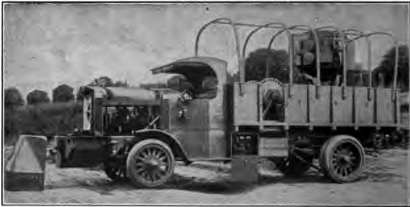
FIG. 9 SEARCHLIGHT EQUIPMENT USED BY ENGINEER CORPS, MOUNTED ON SPECIAL MACK 6-TON CHASSIS
