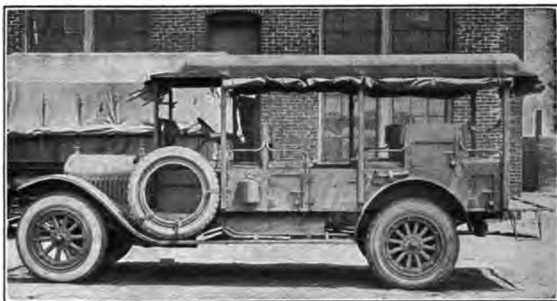
FIG. 1 ARTILLERY RECONNAISSANCE BODY ON \frac{3}{4} -TON CHASSIS
