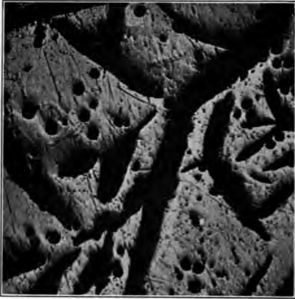
FIG. 2 MICROGRAPH SHOWING FREE CARBON IN CAST IRON
