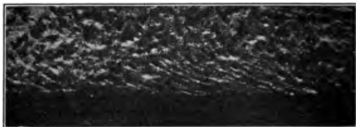
FIGS. 12 AND 13 PHOTOMICROGRAPHS OF THE INNER EDGE OF A BUSHING FINISHED WITH A DULL BROACH (60 MAGNIFICATIONS), SHOWING MUTILATION OF THE SURFACE MATERIAL
