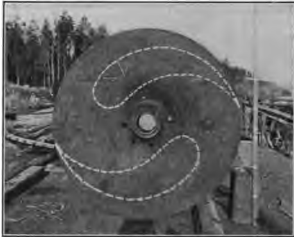
FIG. 9 REAR VIEW OF TWO-VANED IMPELLER DESIGNED BY A. B. WOOD
