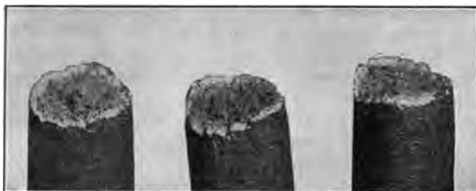
FIG. 13 FRACTURES SHOWING WIDTH OF DECARBONIZED RIM
