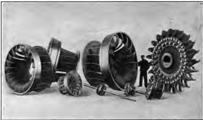
FIG. 2 TYPICAL GROUP OF MODERN MIXED-FLOW, REACTION (FRANCIS) RUNNERS CONTRASTED TO IMPULSE-TYPE WHEEL SHOWN ON THE RIGHT
