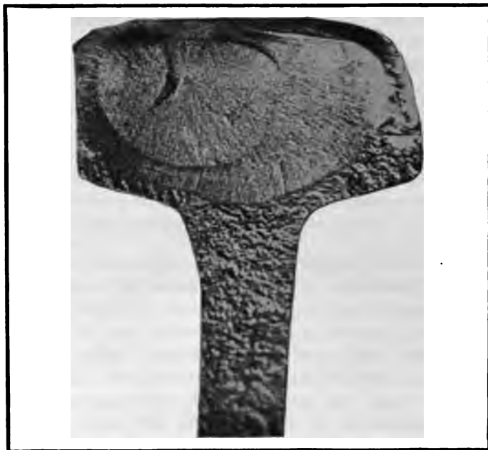
FIG. 21 TENSION FRACTURE IN A STEEL RAIL
