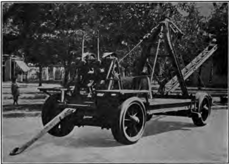
FIG. 6 CRANE FOR ORDNANCE AND ARTILLERY PURPOSES MOUNTED ON 10-TON TRAILER
