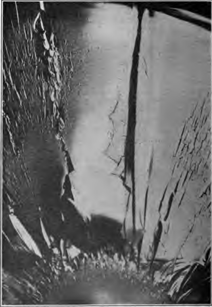
FIG. 9 FRACTURE IN GLASS
