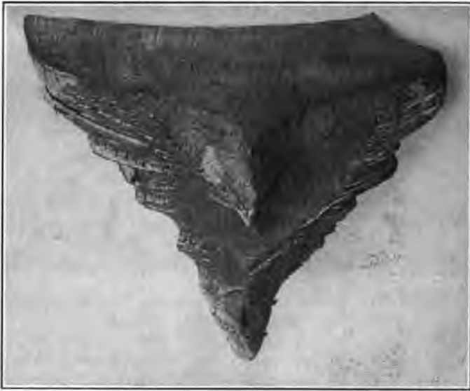
FIG. 19 PIECE OF STEEL TIRE BROKEN IN A DROP TEST
