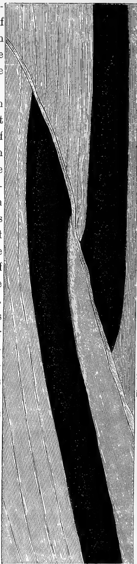
Fig. 10.—Reversed Fault, Brockwell coal, George Pit, Etherley.
