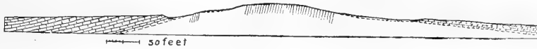
FIGURE 3.—Transverse section of the quaquaversal dome at Fort Hill, Kingston. Horizontal and vertical scales equal.
