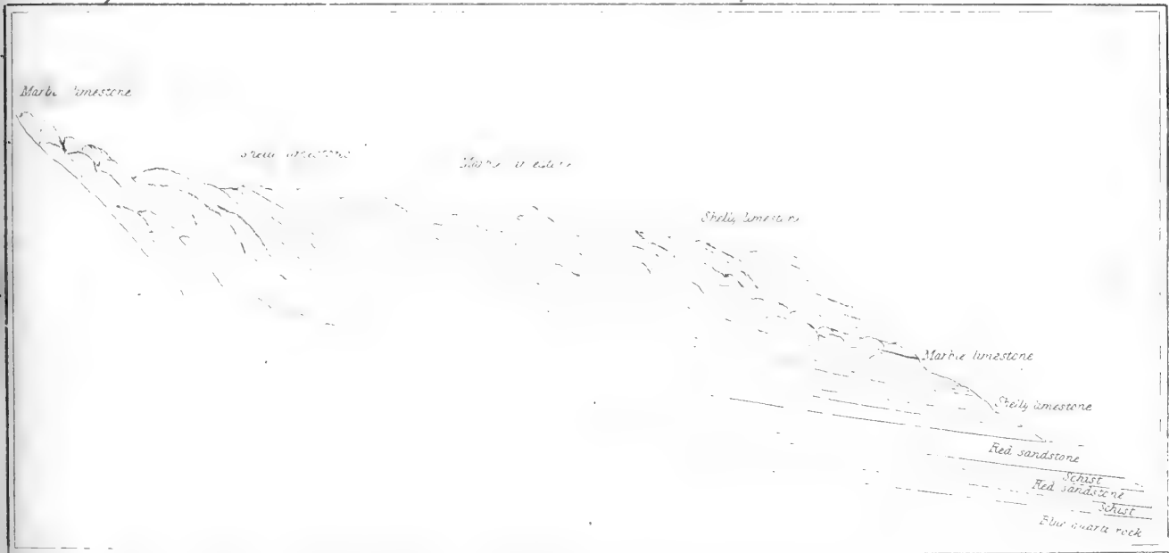
Section of the same in another direction, prolonged towards Berrereg showing the superpositions of the strata, and an example of alternation between the Shelly & the marble limestone
