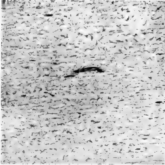
FIG. 2.—Longitudinal section of soft steel plate containing 0.12 to 0.15 per cent. of carbon; etched with picric acid and sodium picrate; magnified 100 diameters.
