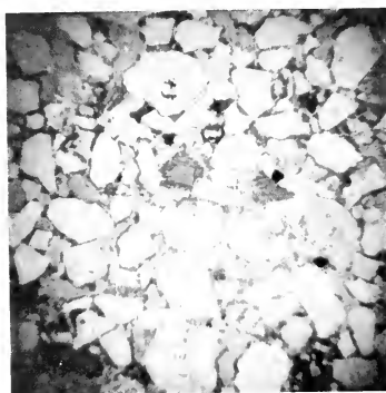
Figure 4. Photomicrograph of Pleistocene Lindavista Fm. sample from Ardath Road locality (magnification 10x). Specimen is a moderately sorted, subangular, medium sandstone with dark cement partially filling the pores.
