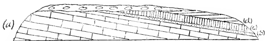
FIG. 2.—Section at Trig. Station Z, Otiake River. (a) Otekaike limestone; (b) glauconitic calcareous bands; (c) less glauconitic calcareous sandstones; with glauconitic bands passing up into (d); (d) softer calcareous mudstone.
