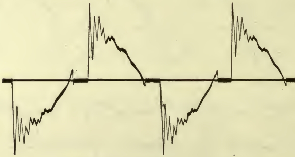
Fig. 77. E.m.f. between rectifier anodes.
