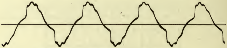
Fig. 68. Secondary terminal e.m.f. of transformer.
