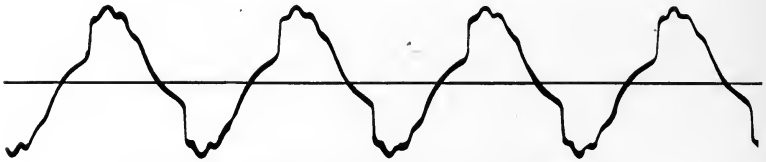
Fig. 68. Secondary terminal e.m.f. of transformer.
