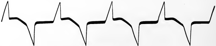
Fig. 69. E.m.f. across a.c. reactive coils.
