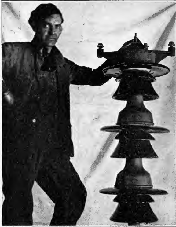
FIG. 109c.—Insulation for 150,000 volt Kilare switch.
