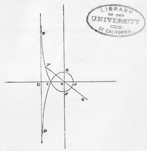
$\theta = \frac{3\pi}{2}$ , r is infinite, and the polar subtangent is 3a, the eye must be supposed at O looking along OF, and a distance OG = 3a must be measured to the right of OF and at right angles to it; a straight line drawn through G parallel to OF is the required asymptote.
