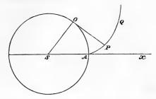
Let S be the centre of a circle, APQ a portion of the involute, OP = OA the portion of the string unwound. Let SO = a,  $OSA = \phi$ , and let x, y be the co-ordinates of P, the origin being at S, and SA the direction of the axis of x.
