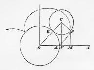
Let O and C be the centres of the fixed and the rolling circles respectively, B the point of contact, P the tracing point, A its initial position. Take OA as the axis of x; draw CN, PM, perpendicular to the axis of x. Let
