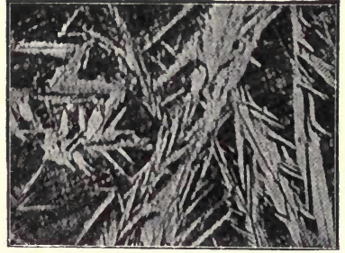
(b) Highly tempered tool steel, rich in carbon; martensite (white needles); austenite (dark, almost formless mass).
