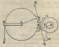
on the circumferences of which the teeth are arranged; C the point of contact of two teeth; QCQ a normal to the surfaces in contact at C. Suppose an axle is fixed on the wheel B, and the weight W suspended from it at E by a cord; also suppose the power P acts by an arm AD; draw Aa, Bb perpendicular to QCQ. Let the mutual pressure at C be Q. Then, since the wheel A is in equilibrium about the fixed axis A, the sum of the moments about A equals zero; therefore
