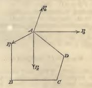
$AP_{2}$ , &c., and join A with the last vertex D, the line AD will represent in magnitude and direction the resultant of all the forces.
