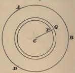
definitely small quantity, then the mass of the circular ring contained between the adjacent circles is  $2\pi\rho\kappa r\delta r$ . Every particle in this circular ring is at a distance  $\sqrt{(a^2 + r^2)}$  from the attracted particle; also the resultant attraction of the ring is in the line through *C* perpendicular to the lamina, and is equal to
