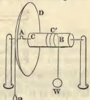
$P \times \text{rad. of wheel} = W \times \text{rad. of axle};$
