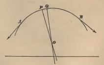
it leaves the curve. Let P, Q be adjacent points in the string; let the normals to the curve at P and Q meet in O; let  $\theta$  be the angle which PO makes with some fixed line, and  $\theta + \delta\theta$ the angle which QO makes with the same line. The element PQ is acted on by a tension at P along the tangent at P, a tension at Q along the tangent at Q, and the resistance of the smooth curve which will be ultimately along PO.
