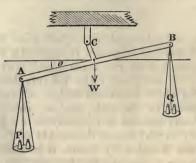
C the fulcrum; h its distance from the line joining A, B: W the weight of the beam and scales: k the distance of the centre of gravity of these (*i. e.* of the point of application of W) from C measured downwards;  $\theta$  the angle the beam makes with the horizon when there is equilibrium.
