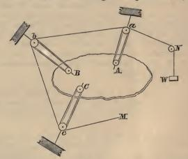
maintain a system in equilibrium; let pullies be fixed to the system at the points A, B, C,... and let the pullies a, b, c,... be attached to fixed blocks, so that Aa may be the direction of the force P, Bb that of Q, and so on. Let a string have a weight W attached to one end, and be passed round the pully N and then round the pullies a and A a sufficient number of times to render the sum of the tensions equal to P. Let the same string then pass on to the pully b, and be passed round b
