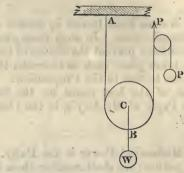
Let the string ABP have one extremity fixed at A, and after passing under the pully at B suppose it held by the hand exerting a force P. The weight W is suspended by a string from the centre C of the pully.
