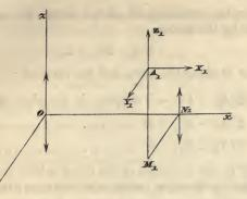
the direction of  $Z_1$  meet the plane of (x, y) in  $M_1$ , and draw  $M_1N_1$  perpendicular to Ox. Apply at  $N_1$  and also at O two forces each equal and parallel to  $Z_1$ , and in opposite directions. Hence  $Z_1$  at  $A_1$  or  $M_1$  is equivalent to  $Z_1$  at O, and two couples, the former having its moment  $= Z_1, N_1M_1$ , and which may be supposed to act in the plane of (y, z), and the latter having its moment  $= Z_1 \cdot ON_1$  and acting in the plane of (z, x).
