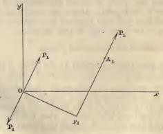
Let  $P_1$ ,  $P_2$ ,  $P_3$ , ..... denote the forces;  $\alpha_1$ ,  $\alpha_2$ ,  $\alpha_3$ , ..... the angles which their directions make with the axis of x; let  $x_1$ ,  $y_1$  be the co-ordinates of the point of application of  $P_1$ ; let  $x_2$ ,  $y_2$  be those of the point of application of  $P_2$ , and so on.
