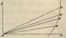
let OP = r,  $POx = \theta$ ,  $POQ = \Delta\theta$ . The area  $POQ = \frac{1}{2}r^2\Delta\theta$ ultimately (*Diff. Calc.*, Art. 313). Also the centre of gravity of the figure POQ will be ultimately, like that of a triangle, on a line drawn from O bisecting the chord PQ, and at a distance of two-thirds of this line from O. Hence the abscissa and ordinate of the centre of gravity of POQ will be ultimately
