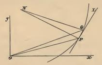
adjacent point; r,  $\theta$  the polar co-ordinates of P; let s be the length of the curve measured from some fixed point up to P, and  $PQ = \delta s$ . Draw PL the tangent at P; and PN, QN normals at P and Q respectively, then PN is ultimately the radius of curvature at P. Let T denote the tension at P,  $T + \delta T$  the tension at Q,  $Fm\delta s$  the force acting on the element PQ, which will ultimately be in the direction OP produced.
