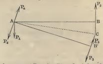
and act on the arm AB. At B' and A let the equal and opposite forces  $P_{s}P_{s}$ ,  $P_{4}P_{s}$ , each equal to  $P_{1}$  or  $P_{2}$  be applied, acting perpendicularly to AB'; this will not affect the action of  $P_{1}$  and  $P_{2}$ .
