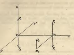
The moment of the first couple is  $P_1y_1$ , and this couple, without altering its effect, may be transferred to the plane of (y, z), which is parallel to its original plane. The moment of the second couple is  $P_1x_1$ , and it is in the plane (x, z).
