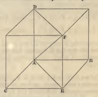
and draw the diagonal AE; then AE represents the resultant of X and Y in magnitude and direction, by Art. 17. Now the resultant of this force and Z, that is, of the forces represented by AE, AD, is represented in magnitude and direction by AF, the diagonal of the parallelogram DE. Hence the resultant of X, Y, Z is represented in magnitude and direction by AF. Let R be the magnitude of the resultant, and a, b, cthe angles the direction of R makes with those of X, Y, Z. Then, since
