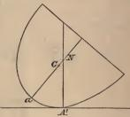
the axis of the parabola further from a than G is, and the equilibrium is *stable*.
