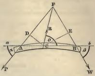
upon the fulcrum, and  $\theta$  the angle which it makes with the line aCb; then if we apply a force R in the direction CR, we may suppose the fulcrum removed, and the body to be held in equilibrium by the forces P, W, R.
