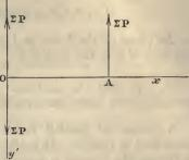
and  $\Sigma P$  acting along Oy' form this couple. The latter force is destroyed by the force  $\Sigma P$  along Oy. Hence the single resultant is  $\Sigma P$  acting at A, that is, at a point the distance of which from O is  $\frac{\Sigma Px}{\Sigma P}$ .
