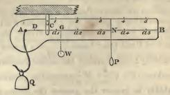
from which the substance to be weighed is suspended, Q being its weight; C the fulcrum; W the weight of the beam together with the hook or scale-pan suspended from A; G the centre of gravity of these.
