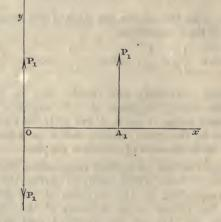
the plane of the forces as origin and draw rectangular axes Ox, Oy, the latter parallel to the forces. Let  $A_1$  be the point where Ox meets the direction of  $P_1$ , and let  $OA_1 = x_1$ .
