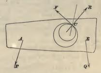
which passes a solid fixed cylindrical axis. Let the outer circle in the figure represent a section of the cylindrical hole made by a plane perpendicular to its axis, and the inner circle the corresponding section of the solid axis. In the plane of this section, we suppose two forces P and Q to act on the solid body at the points A and B. Also at the point of contact C there is a normal force R and a tangential force F. These four forces keep the body in equilibrium.
