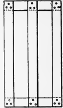
FIG. 245.—Drying lath for tile.
