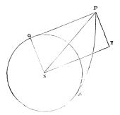
A the point from which the string began to be unwrapped, QP the string once coincident with the arc AQ, and therefore = AQ; PY a tangent to the curve AP or to the involute, SY perpendicular to the tangent, join SP.
