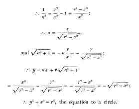
PROB. II. A straight line of given length slides down between two rectangular axes, find the curve to which it is always a tangent.
