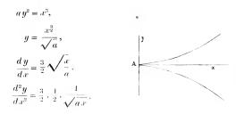
If x = 0, y and  $\frac{dy}{dx} = 0$ , if x = -h, they are both impossible. But if x = h, y and  $\frac{d^2y}{dx^2}$  have two values, one positive and the other negative; the axis of x is therefore a tangent: there are two branches to the curve, one above and the other below the axis of x, and both convex to it, but the curve does not extend through the origin to the negative axis of the abscissas. The origin is a cusp of the first species.
