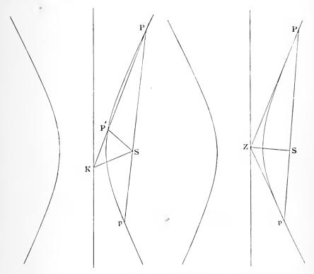
Take a point P' on the hyperbola near to P, and let the chord PP' meet the directrix in K, and produce PS to p. Then KS bisects the angle P'Sp. [Prop. 2.
