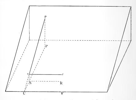
Let ps, sr be two straight lines at right angles to one another, of which sr is parallel to the base line UV. Let PS, SR be their projections. Since sr is parallel to UV, it does not meet the plane of projection PSUV, hence sr does not meet SR; also sr, SR are in the same plane, therefore they are parallel to one another.
