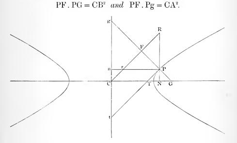
Draw RPN, Prn, perpendiculars on the axes meeting CF in R and r, and let the tangent at P meet the axes in T and t.
