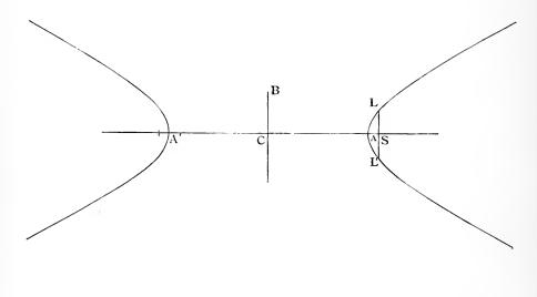
$SL^{2} : AS \cdot A'S = CB^{2} : CA^{2}.$   $AS \cdot A'S = CB^{2},$   $\therefore SL^{2} : CB^{2} = CB^{2} : CA^{2};$   $\therefore SL : CB = CB : CA;$   $\therefore SL \cdot CA = CB^{2}.$ [Prop. 3. [Prop. 3. [Prop. 3. [Prop. 3.]]
