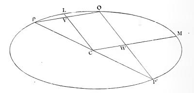
Draw the diameters CL, CM parallel to the supplemental chords P'Q, QP cutting them in V and W.
