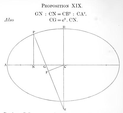
Produce PG to meet the minor axis at g, and draw CF parallel to the tangent at P, meeting Pg at F.
