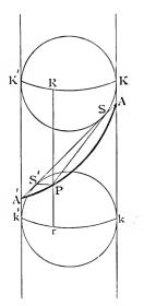
Let APA' be the curve of section. Take the axial plane for the plane of the paper, and let it meet the cutting plane in the straight line AA' and the cylinder in the generating lines KAk, K'A'k'.
