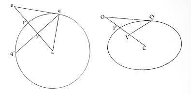
Draw the circle whose projection is the ellipse. Let c, q, o, p, v be the projections of C, Q, O, P, V. Join cq and produce qv to meet the circle at q'.
