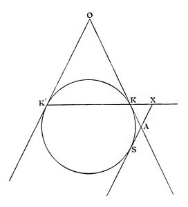
angle AKX = angle OKK'  $\therefore$  = angle OK'K = angle KXA; [Euc. I. 29.  $\therefore AK = AX$ , [Euc. I. 5.  $\therefore SA = AX$ , [Euc. III. 36.
