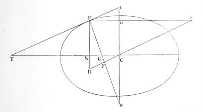
Draw PNR, Pnr perpendicular to the axes meeting CF in R and r, and let the tangent at P meet the axes at T and t.
