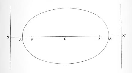
If we take CS' equal to CS, and CX' equal to CX, and through X' draw a line perpendicular to AA', the ellipse can be described with this line as directrix, S' as focus, and eccentricity the same as before.
