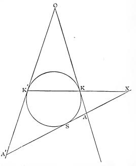
Let the axial plane meet cutting plane in AX, the focal sphere in the circle KK'S, and the cone in the generating lines OKA, OK'. Produce K'K and SA to meet in X the foot of the directrix.
