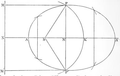
From the focus S draw SX perpendicular to the directrix. Divide XS in A, so that
