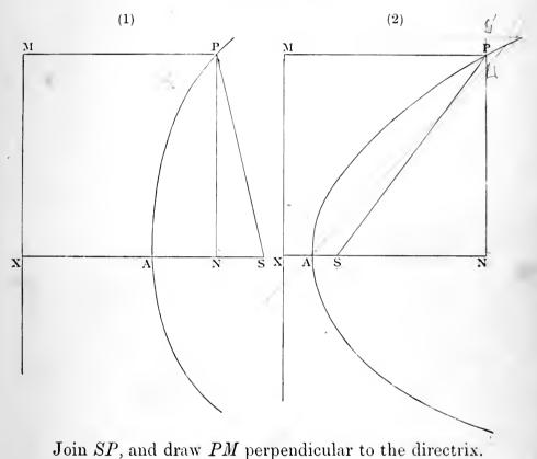
Then, since SA = AX, and AS is divided in N (Fig. 1), AN is divided in S (Fig. 2);  $\therefore NX^2 = SN^2 + 4AS \cdot AN$ . [Euc. II. 8. But  $NX^2 = PM^2$  $= SP^2$
