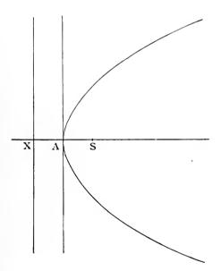
If the point P be at the vertex A, the angle SPM is two right angles and coincides with the straight angle SAX. Hence the tangent, which bisects this angle, is at right angles to the axis.
