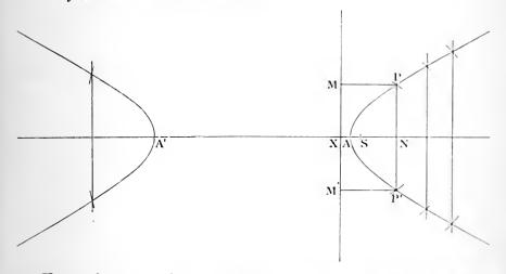
From the focus S draw SX perpendicular to the directrix. Divide XS in A, so that
