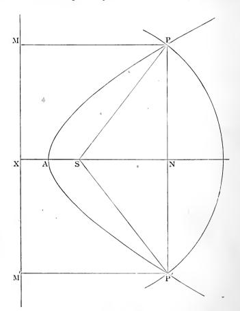
Let S be the focus and MXM' the directrix. Through S draw a straight line SX perpendicular to the directrix, and produce it indefinitely in the direction XS.
