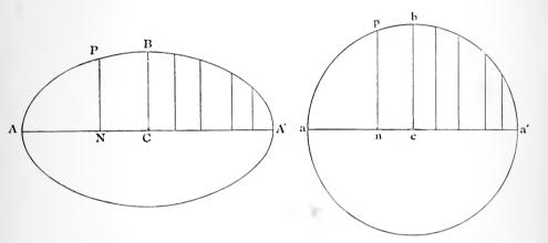
Let apa' be a circle, having its diameter aa' parallel to the base line, cb the radius perpendicular to aa', pn a perpendicular from any point p to aa'.
