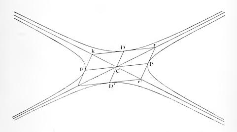
Also the triangle rCr' = parallelogram CPrD, for they are, each of them, a quarter of the parallelogram formed by the tangents at P, D, P', D'.
