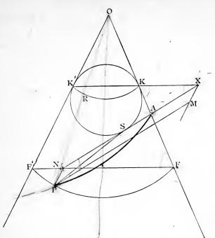
Let AP be the curve of section. Take the axial plane for the plane of the paper, and let it meet the cutting plane in the straight line NAX and the cone in the generating lines OKAF, OK'F'.
