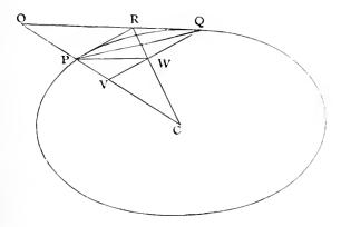
Then  $\because PRQW$  is a parallelogram,  $\therefore RW$  bisects PQ,  $\therefore RW$  passes through the centre, [Prop. 25.  $\therefore$  by similar triangles CV: CP = CW: CR = CP : CO,  $\therefore CV, CO = CP^2$ .
