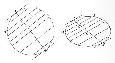
Draw the circle whose projection is the ellipse. The middle points of the system of parallel chords of the ellipse are the projections of the middle points of a system of parallel chords of the circle. [Props.  $\beta$  and  $\gamma$ .
