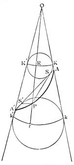
Let APA' be the curve of section. Take the axial plane for the plane of the paper and let it meet the cutting plane in the straight line AA', and the cone in the generating lines KAk, K'A'k'.
