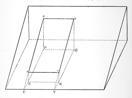
Case 1. Let pqrs be a rectangle, having two sides pq, rs parallel to the base line, and let PQRS be its projection; produce ps, qr to meet the base line in U, V.
