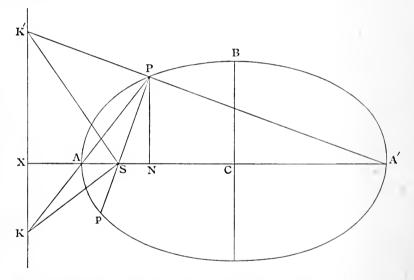
Join PA, A'P, and produce them to meet the directrix at K and K'.
