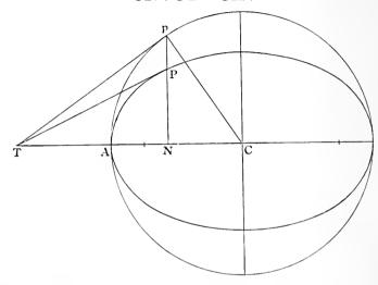
Produce NP to meet the auxiliary circle in p, and join pT, pC.
