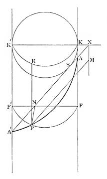
Let APA' be the curve of section. Take the axial plane for the plane of the paper, and let it meet the cutting plane in the straight line  $\dot{A'}AX$  and the cylinder in the generating lines KAF, K'F'A'
