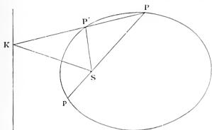
Take a point P' on the ellipse near to P, and let the chord PP' meet the directrix in K, and produce PS to p. Then KS bisects the angle P'Sp. [Prop. 2.
