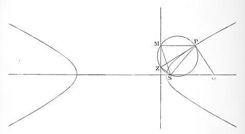
Draw the tangent PZ, join SZ, draw PM perpendicular to the directrix, and join SM.
