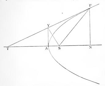
Join SP, and draw PN perpendicular to the axis. Then, since TN is bisected in A, and AY is parallel to PN,  $\therefore PT$  is bisected in Y.
