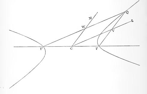
Draw the diameters CL, CM parallel to the supplemental chords P'Q, PQ cutting them in W and V.
