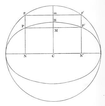
Let pmp' be a chord of the auxiliary circle, cutting the minor axis at right angles in m. Take P and P' points on the ellipse corresponding to p and p', and draw the common ordinates pPN, p'P'N', and join PP', cutting the minor axis in M.
