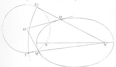
(*Third method.*) With centre O and radius OS describe a circle, and with centre S' and radius AA' describe a second circle intersecting the first in U and U'. Join S'U, S'U'meeting the ellipse in Q and Q', then
