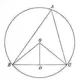
Let O be the circum-centre; draw OD perpendicular to the side BC of the triangle ABC, then D is the middle point of BC, and the angle BOD = A.
