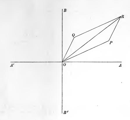
$x_2 + \iota y_2$ , we may therefore express the rule of addition thus; draw from O the straight line OP to represent  $x_1 + \iota y_1$ , and then from P draw PR to represent  $x_2 + \iota y_2$ , join OR, then OR, or the point R, represents the sum  $x_1 + x_2 + \iota (y_1 + y_2)$ .
