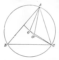
thus O is the centre of the circle round ABC, hence  $OA = \frac{1}{2}a \operatorname{cosec} A$ , or  $h = \frac{1}{2}a \tan a \operatorname{cosec} A$ . When the measurement of the elevation at C is a + n'', let O be the projection of the top of the mountain, then since the elevations at A and B are equal, OO' is perpendicular to AB; let h + x now be the height of the mountain. We find geometrically,
