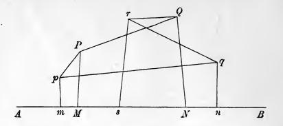
to the projection of PQ on AB. For the sum of the projections is Mm + mn + ns + sN, which is, according to Art. 14, equal to MN. We obtain thus the fundamental property of projections. The sum of the projections on any fixed straight line, of the parts of any broken line joining two points P and Q, depends only upon the positions of P and Q, being independent of the manner in which P and Q are joined.
