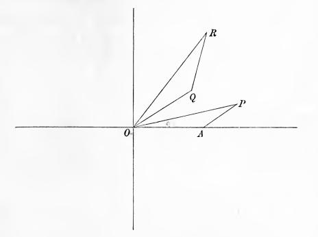
$x_1 + \iota y_1, x_2 + \iota y_2$ ; join AP, on OQ describe a triangle QOR similar to AOP, and so that the angle QOR is equal to  $+\theta_1$ , then  $ROA = \theta_1 + \theta_2$ , and also OR : OQ :: OP : OA, hence the length of OR is equal to the product of the lengths of OP and OQ; it follows that the point R represents the product  $(x_1 + \iota y_1)(x_2 + \iota y_2)$ . 15-2
