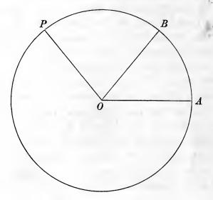
whose length is equal to the radius of the circle; we shall shew that the angle AOB is of constant magnitude independent of the particular circle used; this angle is called the *Radian* or unit of circular measure, and the magnitude of any other angle is expressed by the ratio which it bears to this unit angle, this ratio being called the *circular measure of the angle*.
