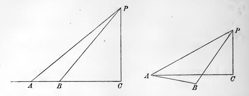
on the horizontal plane, if possible so that ABC is a straight line; let the elevations of P at A and B be measured, denote them by  $\alpha$  and  $\beta$ ; then  $a = AC - BC = h (\cot \alpha - \cot \beta)$ , therefore
