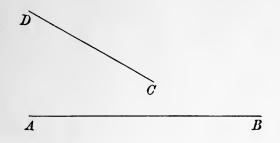
bounding lines. It follows, that if AB, CD are the positive directions in two straight lines, the angle between AB and DC differs by two right angles from the angle between AB and CD, for a line revolving from the position AB, must turn through an angle in order to coincide with DC, 180° greater or less than the angle it must turn through in order to coincide with CD.
