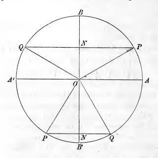
sign, and the projections of OP and OQ, on OB, are equal and of the same sign, therefore  $\sin(\pi - \alpha) = \sin \alpha$ , and  $\cos(\pi - \alpha) = -\cos \alpha$ . These equations hold whatever  $\alpha$  may be, so that we can change  $\alpha$ into  $-\alpha$ , and we have
