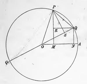
make angles A, B, respectively, with OA; join PQ, and draw PM, QN, perpendicular to OA, and QR parallel to OA, then we have
