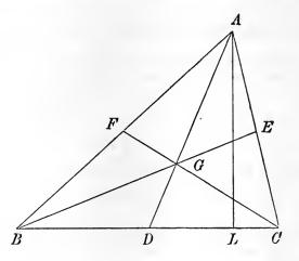
*medians.* The length of AD is given by the well-known geometrical theorem  $AB^2 + AC^2 = 2(AD^2 + BD^2)$ , thus the squares of their lengths are given by
