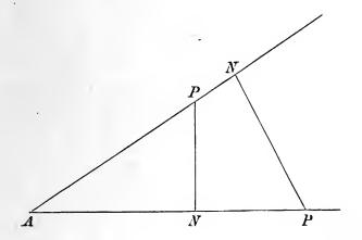
be any point in either of the bounding lines of the given angle; draw PN perpendicular to the other bounding line, we have then
