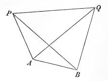
both visible from each of them. At A measure the three angles  $PAQ = \alpha$ ,  $QAB = \beta$ ,  $PAB = \gamma$ ; it should be observed that the angles PAQ, QAB, are in general not in the same plane. At B measure the angles  $PBA = \delta$ , and  $QBA = \epsilon$ .
