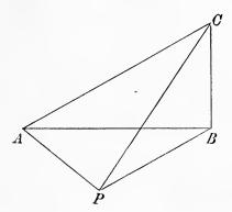
Let  $\alpha$ ,  $\beta$ , be the angles subtended by the sides AC, CB, of a triangle ABC at the point P, and let x, y, denote the angles PAC, PBC respectively; the position of P is found when the angles x and y are determined, for the distances PA and PBcan be found by solving the triangles PAC, PBC.
