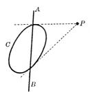
AB, and is called the polar line of P and the conic. If P is within the conic,  $g_y = 0$  joins the imaginary points of contact of the tangents to C from P.
