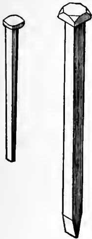
FIG. 126. CUT SPIKE. FIG. 127. BOAT-SPIKE.
