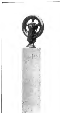
Fig. 503.—Pulley arranged on broom-handle to be fastened at foot of bed for carrying extension cord.
