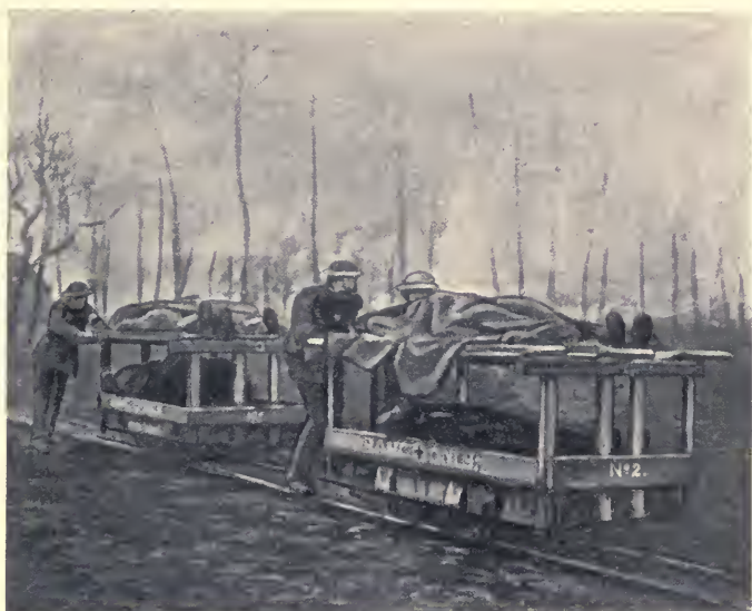
Fig. 5.—Light railway ambulance trolley (redrawn). (Kindness of the editor of the British Medical Journal and of Sir A. A. Bowlby, Bart. See Prefatory Note.)
