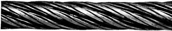
Fig. 7. Lang-Lay Traction Rope as it appeared after having transported over 660,000 tons of ore.
