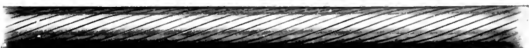
Fig. 3. Trenton Locked-Coil Track Cable ( 1\frac{1}{4} inch diam.), from the Highland Boy Tramway, Bingham, Utah, after carrying two million tons of ore in a period of 6 years. (From photographs.)
