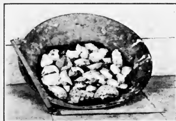
FIG. 62.—Chunks of amalgam from Hardinge amalgamator.
