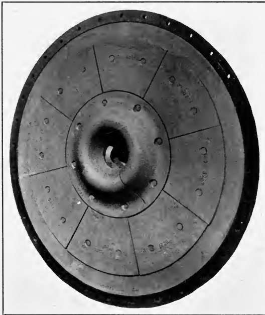
FIG. 35.—Feed head lining of 5 by 8-ft. tube mill at the United Gold Mines Co. mill, Oregon.
