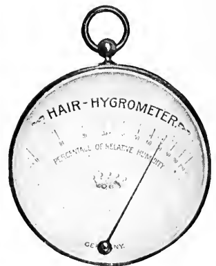
FIG. 42.—HAIR HYGROMETER REGISTERING DIRECTLY RELATIVE HUMIDITY.
