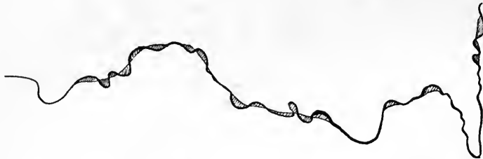
Napier-Wairoa road, showing curves straightened by H. B. C. C.
