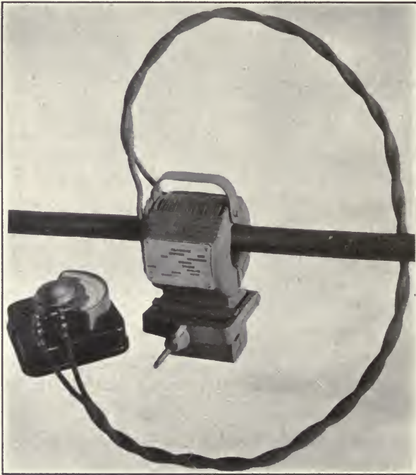
FIG. 156.—Split-core cable-testing transformer.
