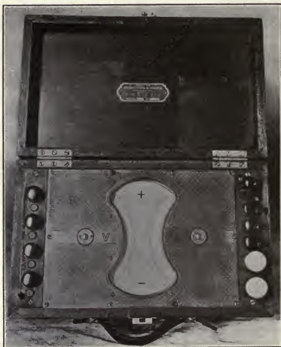
Fig. 146.—Weston duplex electrolysis instrument.
