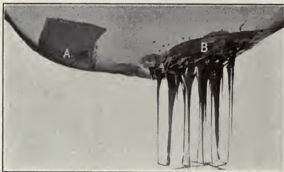
FIG. 79.—Viscosity test of cable-sleeve-filling compounds.
