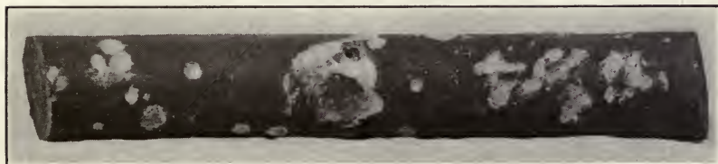
FIG. 144.—Cable damaged by electrolysis.
