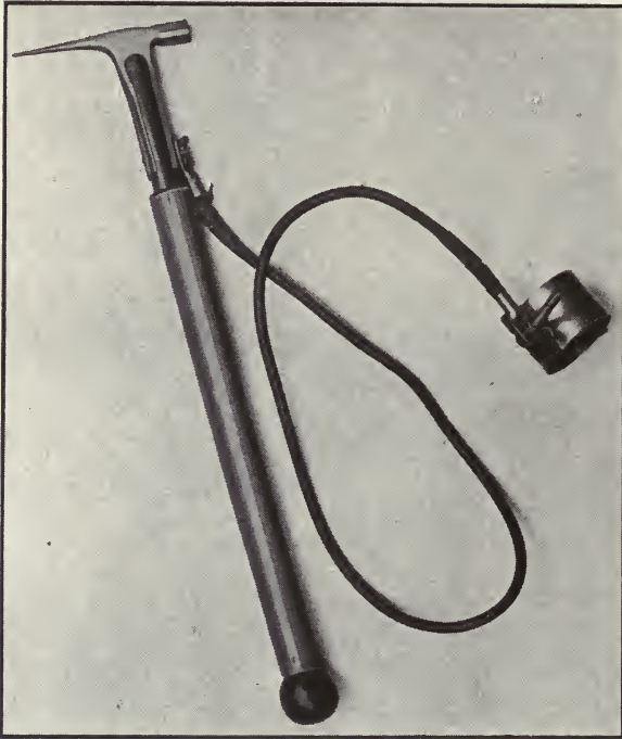
FIG. 106.—Tool for testing cable.
