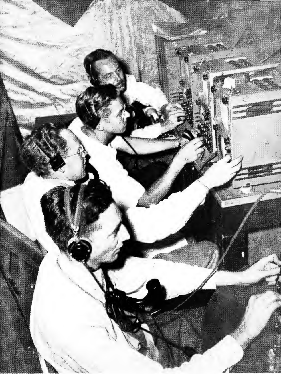
Control operators inside the telemobile station monitor the pictures of field events before the scenes are relayed to the main television station.
