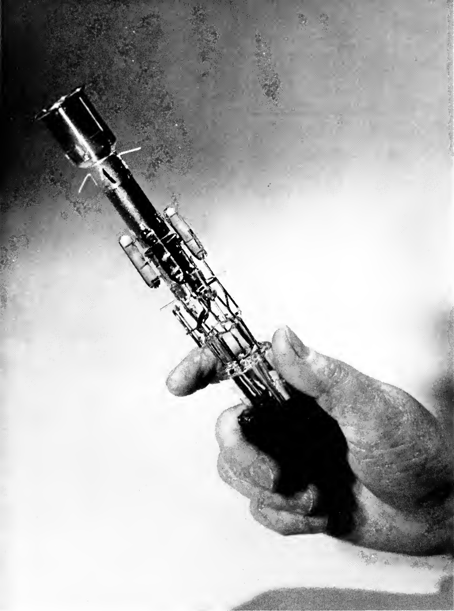
The electron gun, when sealed in the tubular neck of the kinescope, generates the pencil-like electron beam, or television "paint brush", which sweeps with incredible speed across the fluorescent face of the tube to "paint" the picture.
