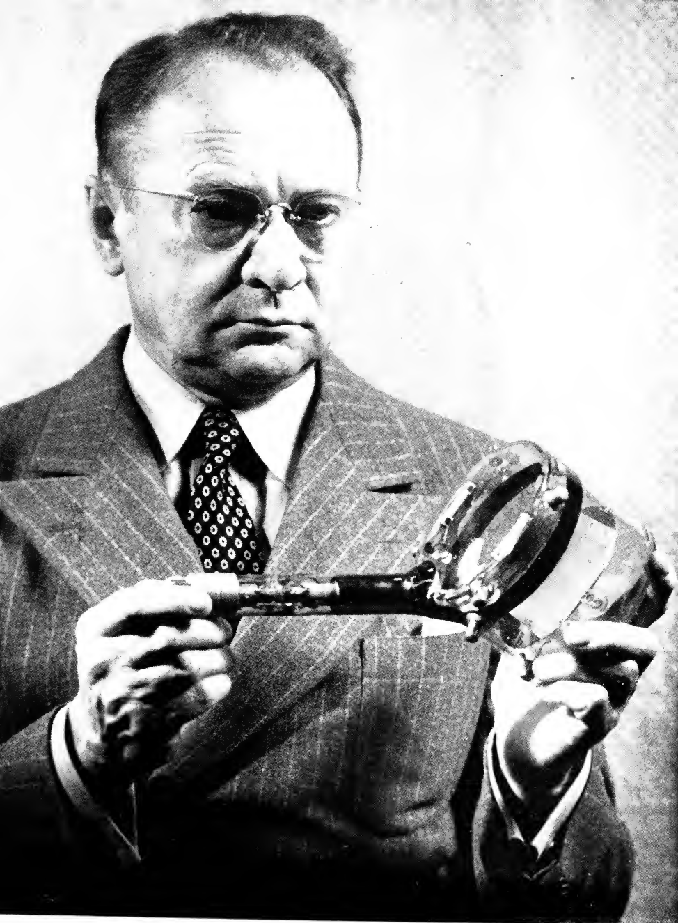
Dr. V. K. Zworykin of RCA Laboratories holding the iconoscope, which he invented as the "eye" of the all-electronic television camera.
