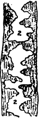
Fig. 10.—Section of vein composed of quartz (1) and calcite (2), from which the calcite has been removed by acid.
