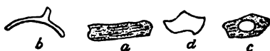
Fig. 15.—Fragments of volcanic glass in tuff as seen under the microscope, \times 50 .
