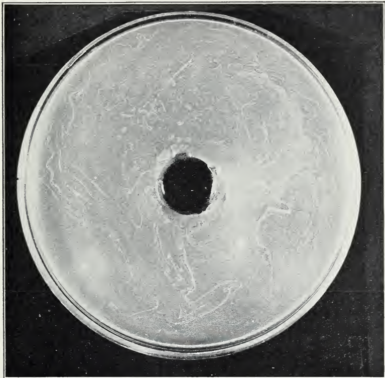
FIGURE 5.—Agar cup-plate method; no antiseptic properties; colonies grow to edge of cup
