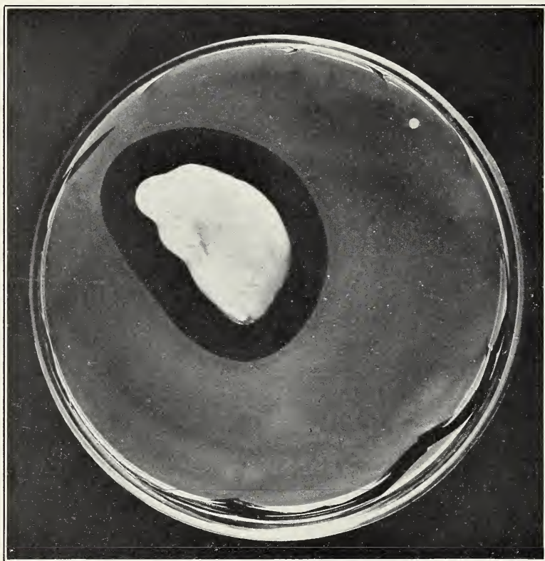
FIGURE 2.—Agar-plate method showing good antiseptic inhibitory properties and good diffusion (dark zone)
