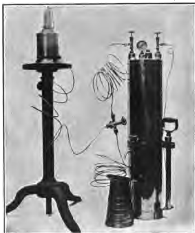
Incandescent oil-vapor lamp, 55-millimeter mantle, with single tank.
