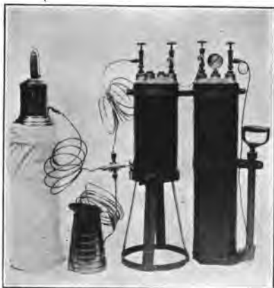
Incandescent oil-vapor lamp, 35-millimeter mantle, with double tanks.
