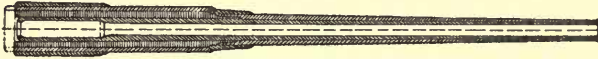
Longitudinal section of a 12-inch gun, showing the number of sections or tubes and hoops of which it is built up.
