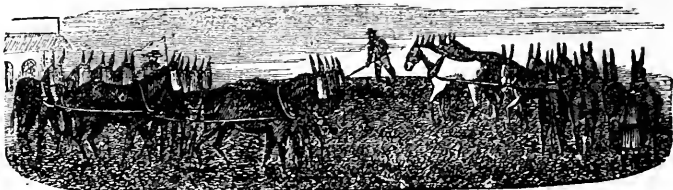
Fig. 34.—AMALGAMATION BY PATIO PROCESS.
