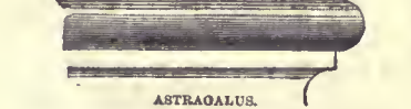
Arch.: "A small semi-circular moulding or Bead, sometimes termed Roundel." (Gloss. of Architecture.)
