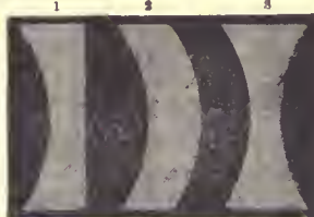
CONCAVE LENSES. 1. Plano-concave. 2. Concavo-convex. 3. Double concave.
