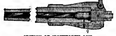
SECTION OF WHITWORTH GUN. b. Reinforce band; c. Breech-block; k. Carriage chamber.
